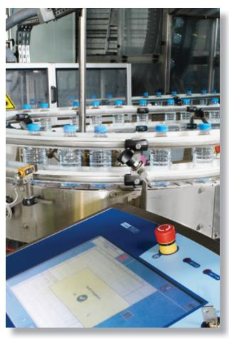
On the multi-format line, Eaux de Chorges uses 7031S laser coder to code two lines of text on the bottle neck.
